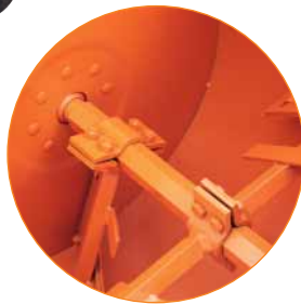
A single piece of 1.63" hex steel makes up the MBW main shaft. Machining, rather than welding or bolting, improves strength and durability. Blade arms are held to the main shaft with conforming plates and hardware.
