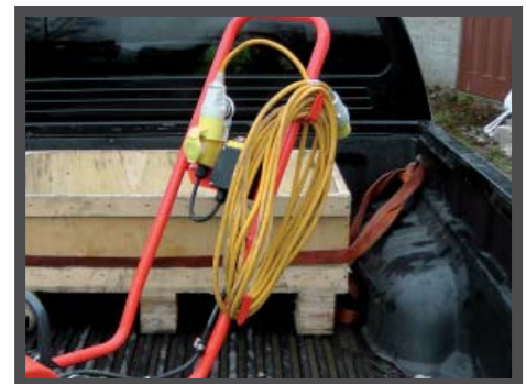
CABLE STORAGE HOOKS ON THE OPERATOR HANDLE
